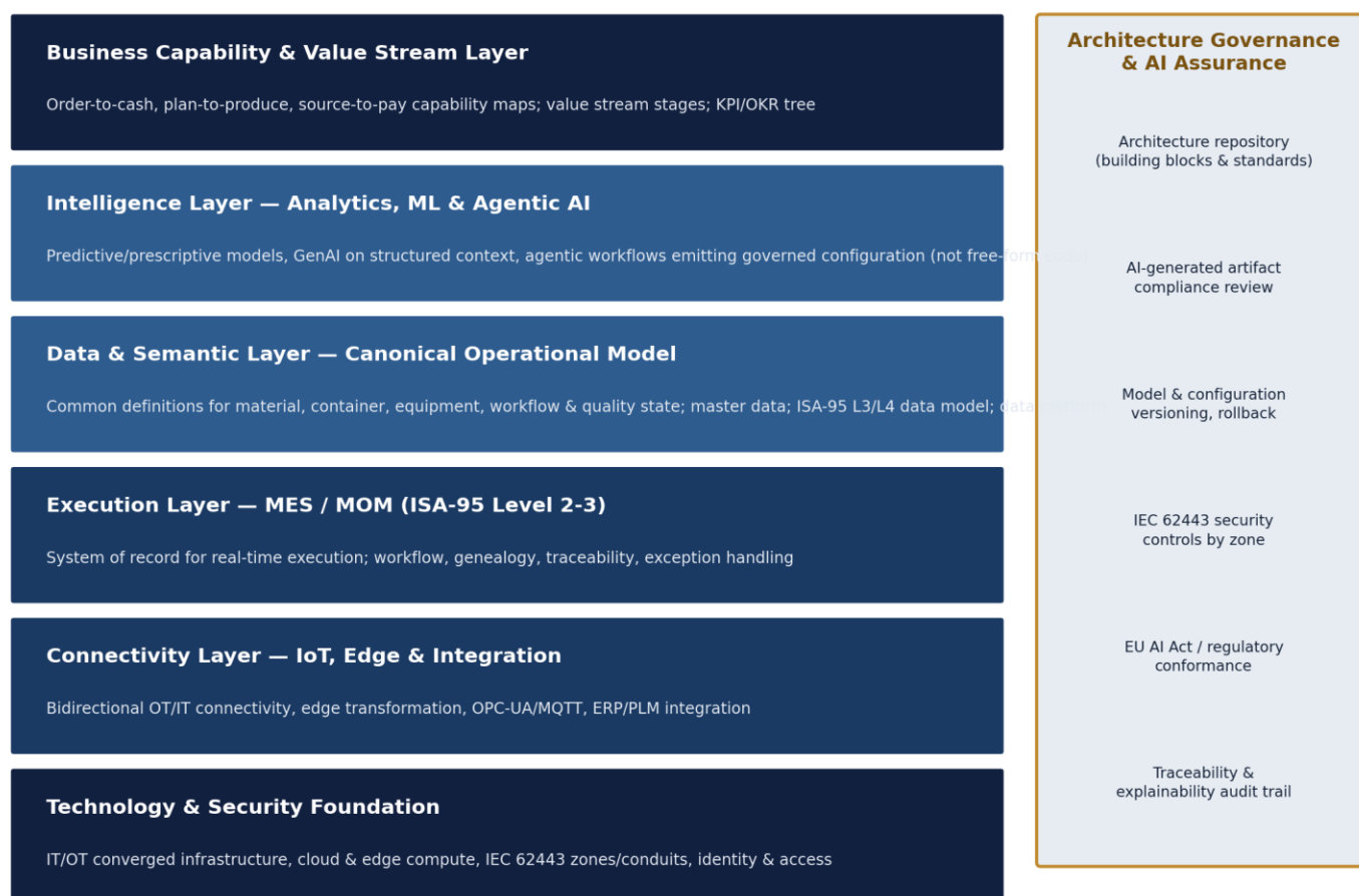
Figure 3. The Industrial AI Operating Model: a vendor-neutral layered reference architecture. Any Industrial Operations Platform, MES, or analytics stack can be mapped onto this structure; the structure itself, not the vendor choice, is the durable enterprise asset.
